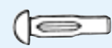
"T" head cotter used extensively in chain industry in place of cotter pins.
